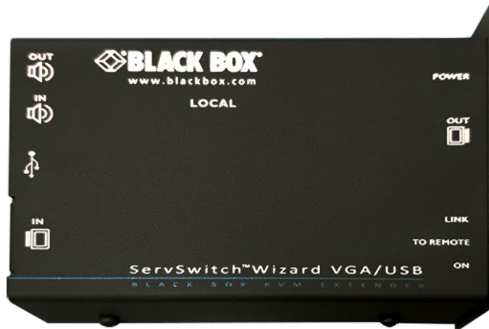
MODEL 5538 BLACK BOX KVM CONNECTIONS (ACU5050A-R2)
