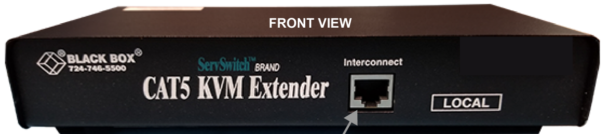
RJ45 Interconnection Cable from Local KVM to Remote KVM
