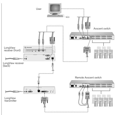
Figure A.3: LongView Installation Example with Multiple Avocent Switches
