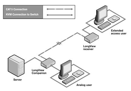
Figure 1.1: A Typical LongView Configuration
