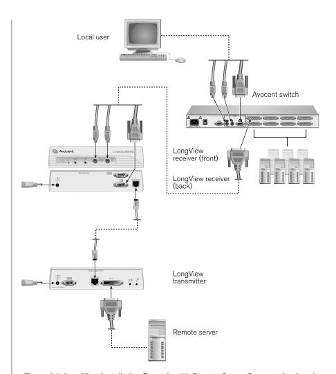
Figure A.2: LongView Installation Example with Remote Server Connected to Local Avocent Switch
